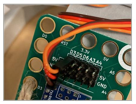
Connect the motor to D3 as shown. You can wind the wire around the structure a few times first so that it takes up the slack.
