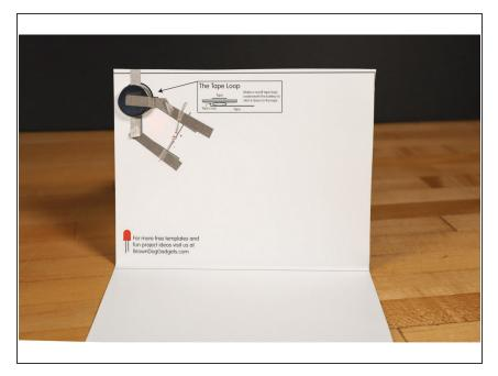
Follow the circuit guide printed on the card. Attach LEDs, a battery, and connect it all together with conductive Maker Tape.
