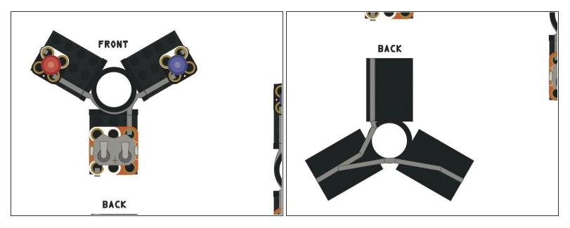
• Start by making sure the parts fit onto the 3D printed studs, both with and without tape. If they're too loose or way too tight, change your print settings and try again.
