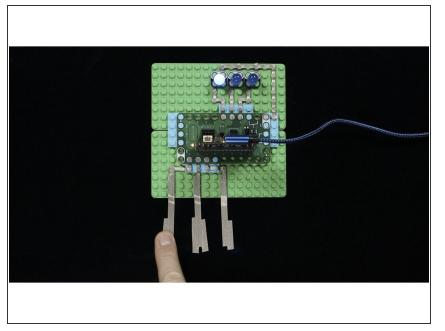
Once you've got your circuit complete and the micro:bit programmed and powered by a USB cable you should be able to touch the Maker Tape to see an LED turn on.
