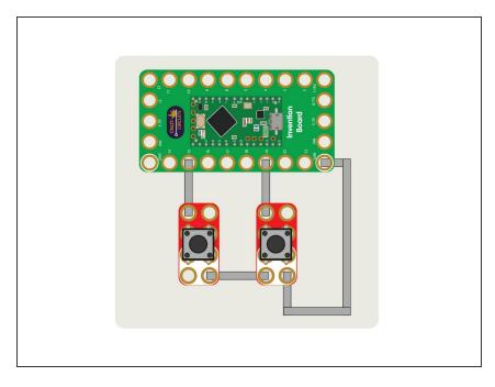
Use a LEGO baseplate to determine the layout of your circuit. You'll need space for the Invention Board, two Jumbo Pushbuttons, and Maker Tape to connect it all together.
