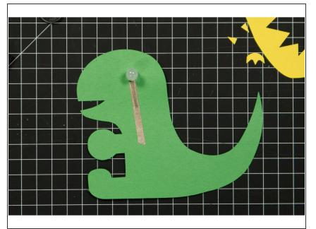
Run a piece of tape along the front of your T-Rex, covering the negative LED leg.
