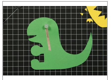
Run a piece of tape along the front of your T-Rex, covering the negative LED leg.
