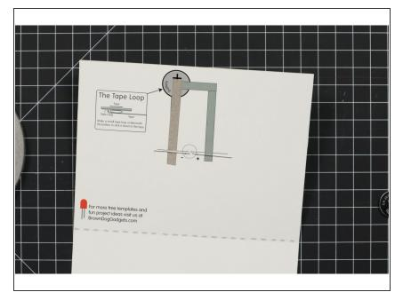
Add a strip of Maker Tape that goes over the negative LED leg and covers about half of the illustration of the battery.
