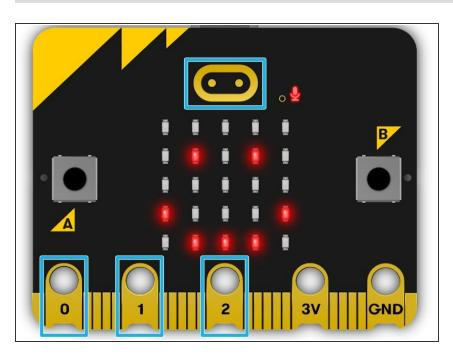
The micro:bit has touch sensors built in to pins 0, 1, 2 (and the logo in the case of the micro:bit v2). The Maker Tape in the foot provides an electrical connection to the touch sensors, so when you touch the foot, those sensors are triggered!
