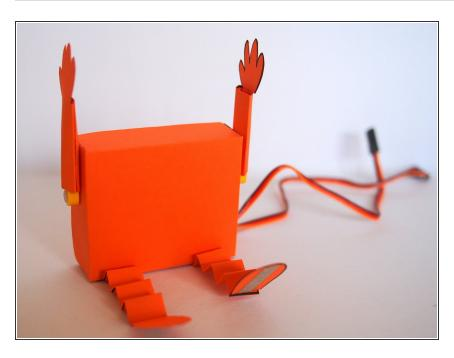
Slide the arms onto the LEGO axle mounts.
