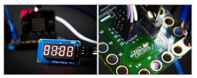
Connect the 7 Segment Display: CLK to Pin 14, DIO to Pin 13, VCC to the + (positive) column, and GND into the - (negative) column.
