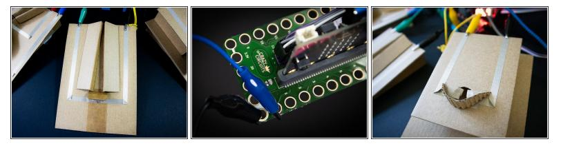
Using alligator clips, connect one side of each switch to ground, and the other to pin 0, 1, 2, and/or
