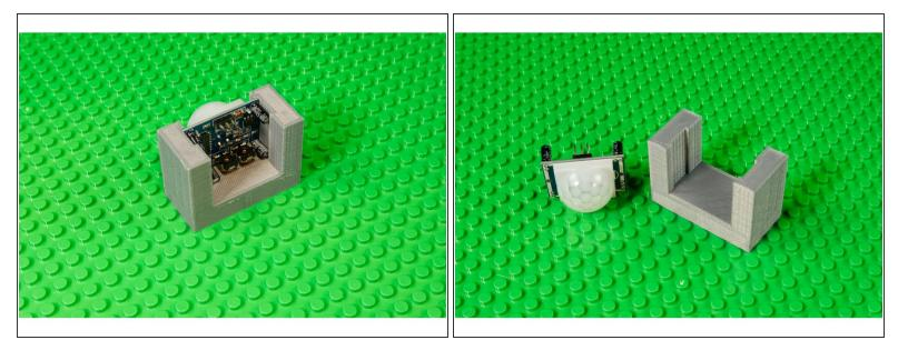
• The PIR Sensor slides into the holder and is held in place by gravity.
