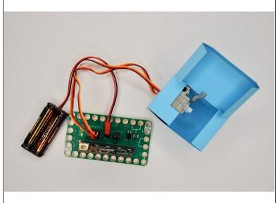
Connect the servos to the Bit Board to Servo Pins 0 and 1.
