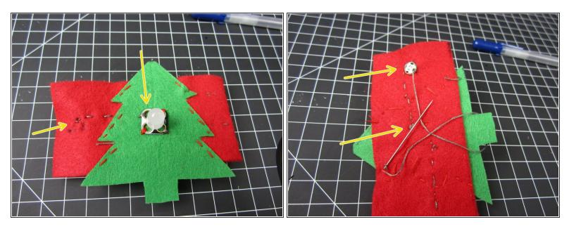
Using Conductive Thread connect one of the white holes on your LED to the other button snap on the opposite side of your fabric.
