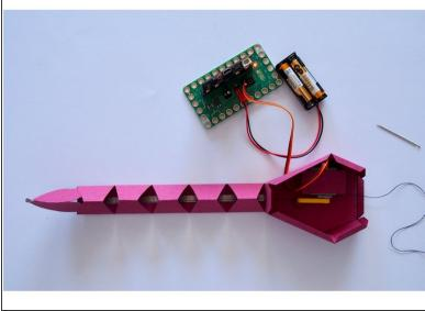
• Tie the string to the end of the LEGO Beam in such a way that it is lightly tensioned when the mount faces towards the tail, and tight enough to pull the tail up when the beam points away from the tail.
