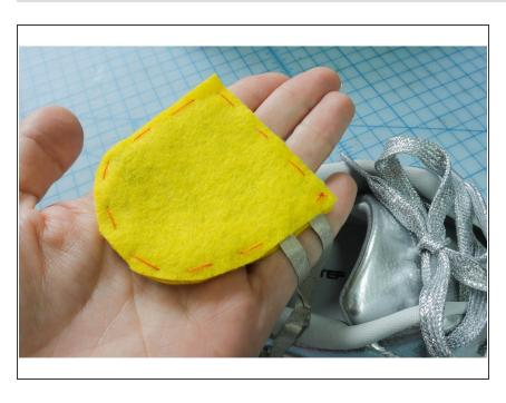
With the sensor laid out correctly, use a needle and thread to stitch around the sensor to keep it together as shown.
