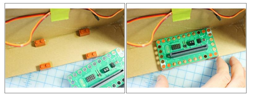
Use super glue to glue 4 small LEGO pieces into place. This will make a resting spot for the Bit Board that will allow it to be easily removed.
