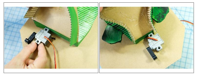
• Thread the motor wires through the holes.
