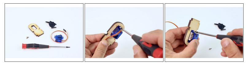
• Using the **wooden servo plate** shown, and the **two matching small screws** found in the last servo bag, **mount the remaining servo** using your Phillips head screwdriver.
