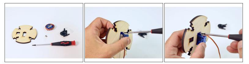
• Using two of the **matching screws** (found in each servo bag) and a small Phillips head screwdriver, **mount one of the servos** as shown onto the circular Solar Tracker platform.
