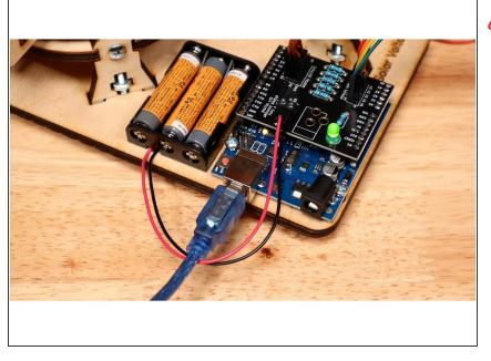
Note: You must power the Arduino via USB and power the shield with the 3 AAA Battery Pack with fresh batteries.
