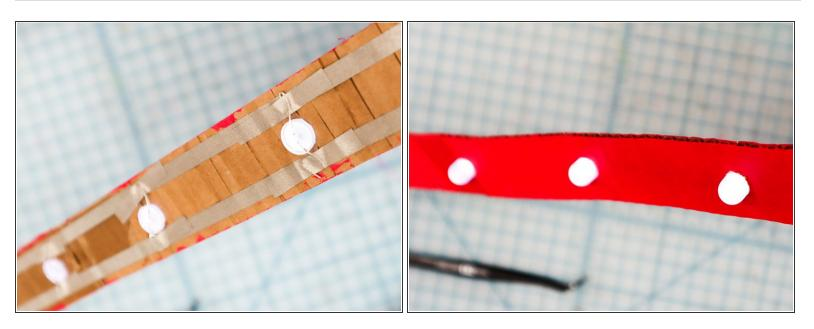
Repeat the previous steps until you have all the LEDs attached to the belt.
