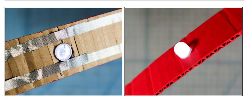
Now, add an extra piece of Maker Tape on top of the LED legs. This should "sandwich" the legs in between two pieces of Maker Tape and the LED should light up!
