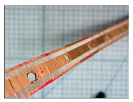
Adhere two strips of Maker Tape to the back of the belt between the edge and the holes. Make sure that the two pieces don't touch each other.
