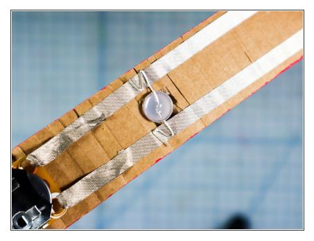
Tuck the LED legs into the belt by folding them back and forth as shown. We've found that this makes a more reliable connection to Maker Tape than cutting the legs.
