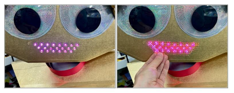
Cover the mouth with a sheet of rhinestones, cut to the shape of a mouth. Remove the mirror backing sheet if you'd like to see the LEDs shine brighter.
