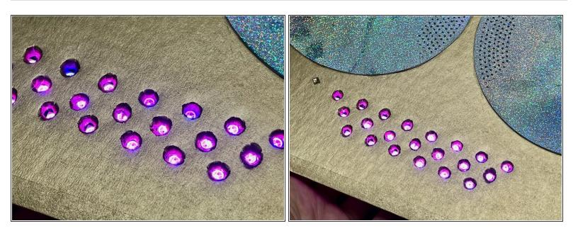
• Use strong tape or hot glue to position and attach the LEDs (and the cardboard they are glued to) behind the holes.
