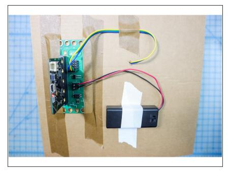
Connect a battery pack to power the circuit on the go.
