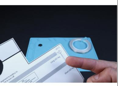
Flip your project over to the circuits side. Bend the LED legs in the directions shown on the diagram so they lay flat against the paper.
