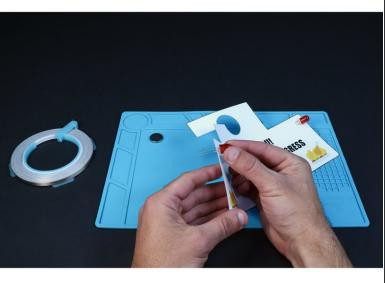
Each of the pairs of holes you just poked is for a single LED. From the front, thread the legs of each of your two LEDs into one of those pairs of small holes. Take care to insert the long LED legs into the upper holes and the shorter LED legs into the bottom holes.
