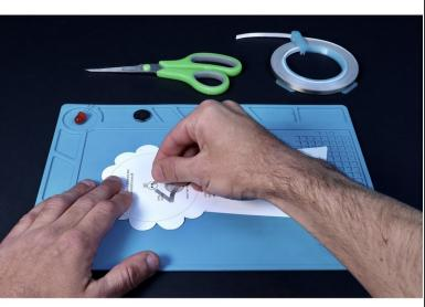
Flip your project to the circuit diagram side. Use a thumbtack or pushpin to poke two holes for the LED legs where shown on the diagram with small black dots.
