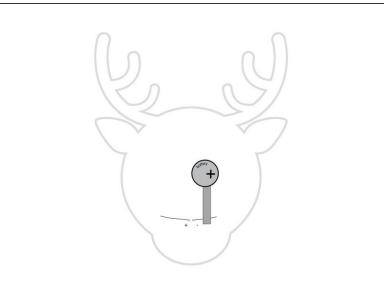
Add a tape loop to the negative piece of tape, then stick the battery down to it. (Make sure you stick the negative side of the battery down.)
