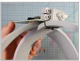
Use a plastic-covered twist tie to attach the servo motor through the GND and 3V holes.
