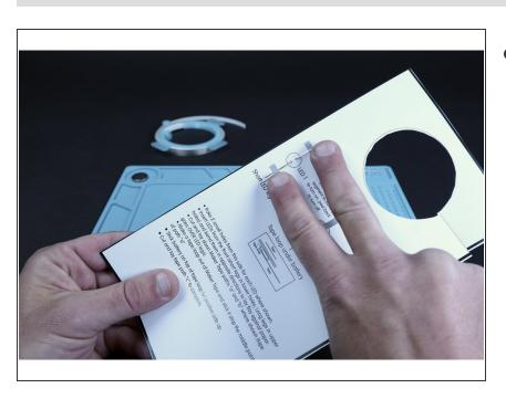
Flip your project over to the circuits side. Bend the LED legs in the directions shown on the diagram so they lay flat against the paper.
