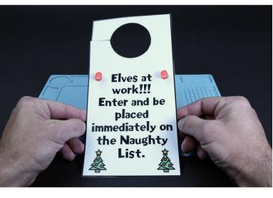
Peel and stick the final Maker Tape pathway where pictured. Sticking it to the top of the battery will turn the LEDs on the opposite side ON, while peeling it back will turn the LEDs OFF.
