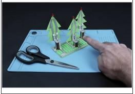
Measure, cut, peel and stick tape paths that lead from the ends of the existing left LED leg paths, down their respective trunks and to their corresponding short segments from the previous step.
