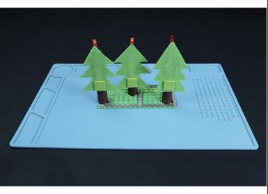
Measure, cut, peel and stick one final tape length where shown so that it can be stuck to the top of the battery. This will complete the circuit and turn on all three of your blinking LEDs. Peeling it away from the top of the battery will turn the circuit off.
