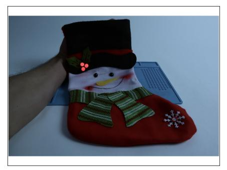
TIP: Oftentimes a circuit gets jostled out of working condition when the stocking is turned right-side-out. The LED may flicker or not work at all. If you encounter this issue, try pressing/firming up every connection point within the circuit where either an LED leg meets the tape OR where one piece of Maker Tape is connected to another!
