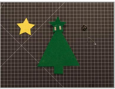
Bend the LED legs down and press them against the tape pads that were added in the previous step.
