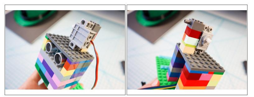
On top of the distance sensor, add another layer of LEGO to mount the servo motor. Use the LEGO Brick 2 x 2 with Pins and Axlehole (30000 / 65514) to mount the motor on its side, as shown.
