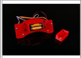
The battery pack sits inside the holder loosely. If you want a more secure fit you can add some tape to hold the battery pack in place.
