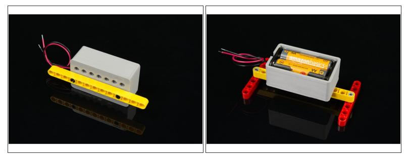
• The battery pack sits inside the holder loosely. If you want a more secure fit you can add some tape to hold the battery pack into place.
