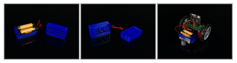
• The battery pack sits inside the holder loosely. If you want a more secure fit you can add some tape to hold the battery pack in place.
