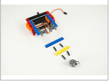
• There are two more beams to attach, each using two pins, and then we can add the caster wheel to the back of the rover.
