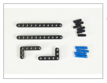
We'll use two long beams to connect the servos together into a frame, and then two L-shaped beams to stabilize the frame a bit more.
