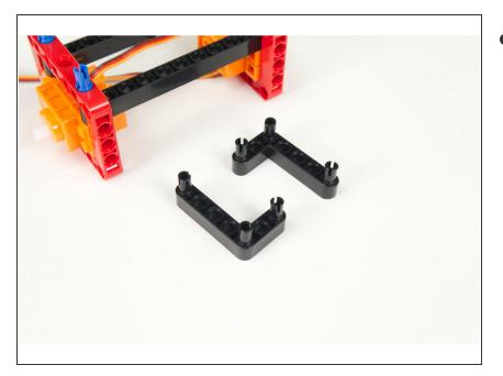
Place pins at the ends and the corner of the two L-shaped beams as shown.
