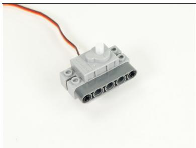
Attach a gray 5 beam to the pins on the servo.
