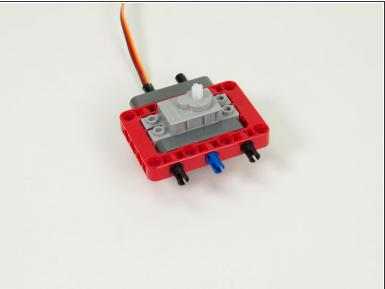
Add two pins to the front of the frame piece as shown.
