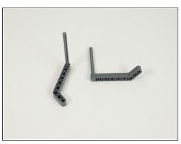
Start the assembly of the "fingers" by sliding the axles into the end of the gray angled beams as shown.
