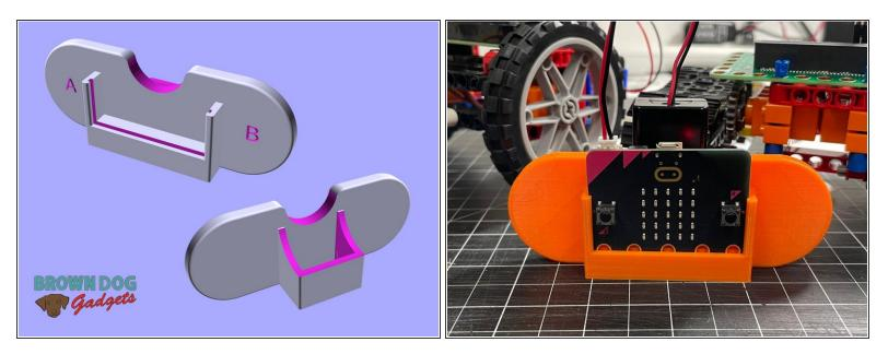
If you find holding the micro:bit and battery pack a little awkward, we've designed a 3D printed holder for you. Check out the: <u>micro:bit Holder</u>
