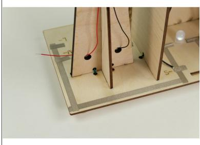
The wires attached to the motor will get connected in front of the windmill, so we'll thread the wires through the holes as shown.
