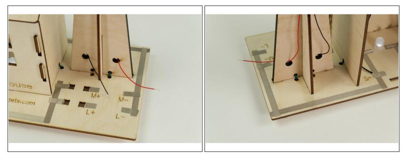
• The wires attached to the motor will get connected in front of the windmill, so we'll thread the wires through the holes as shown.
