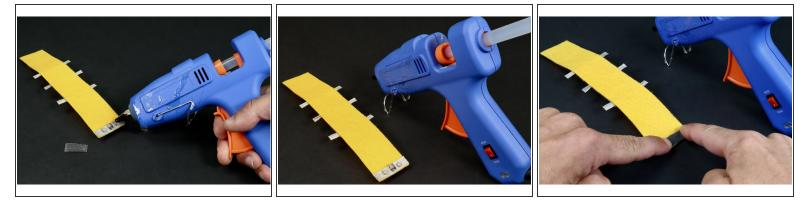
Continue by hot gluing the remaining portion of the conductive hook and loop on top using two dots of glue on either side of the tape loop. Remember: do NOT add hot glue on top of the loop...only the areas to the right and left of it.
