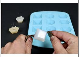
Attach the last LED to the cardboard/tape and make/remove a third & final jewel using the same process that you did for the first two.
