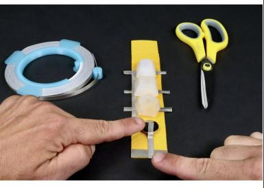
Measure, cut, peel and stick another Maker Tape segment that reaches from the top of the battery all the way to the two overlapping pieces from the previous step.
