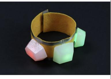
Your bracelet is now complete! To complete the circuit and turn the bracelet on, simply connect the conductive hook and loop.
