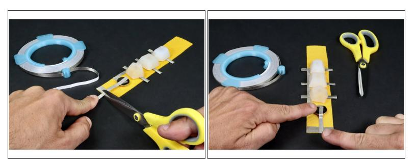
• **Measure, cut, peel and stick** another Maker Tape segment that reaches from the top of the battery all the way to the two overlapping pieces from the previous step.
