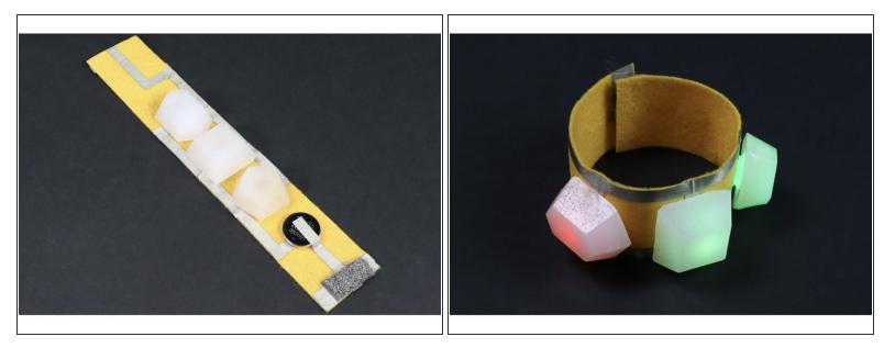
• Your bracelet is now complete! To complete the circuit and turn the bracelet on, simply connect the conductive hook and loop.
