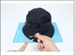
• Cut two small pieces of Maker Tape and sandwich the metal ends of each of the two wires leading from the battery pack just as you had each of the individual LED legs earlier. The black wire is negative and the red wire is positive.
