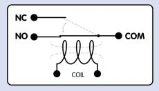
COM is connected to Normally Open when the coil is energized.
