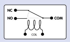
COM is connected to Normally Closed when the coil is not energized...
