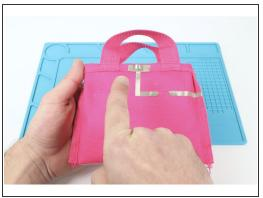
Cut three small pieces of Maker Tape and turn them into three tape loops, placing them afterward atop your existing Maker Tape paths where shown at left and in step 6 of the featured document.
