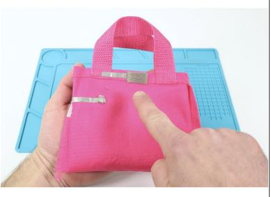
Using one of the three methods described in our Conductive Hook & Loop guide (included at the end of the featured document), attach Conductive Hook on one side atop one of the upper Tape Loops and the Conductive Loop atop the remaining upper tape loop.
