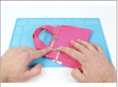
Stick a CR2032 battery positive (+) side UP atop the remaining lower tape loop. Then measure, cut, peel and stick a final Maker Tape path connecting the top of the battery to the Maker Tape path above the battery as shown.
