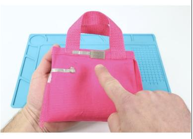
Using one of the three methods described in our Conductive Hook & Loop guide (included at the end of the featured document), attach Conductive Hook on one side atop one of the upper Tape Loops and the Conductive Loop atop the remaining upper tape loop.
