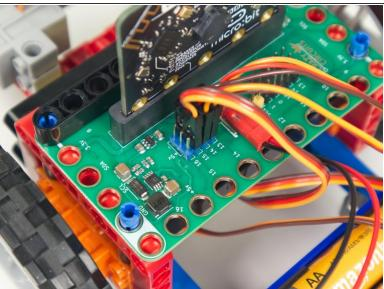
Plug the servo connector into the row for Pin 15. The orange wire should go to the pin closest to the 15 on the board, the red wire goes into the +5v row, and the brown wire goes into the - row, which is ground.
