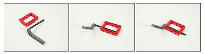
• Slide the axle (with the beam attached) into the red frame.
