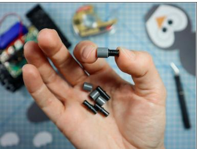
Connect each LEGO pin to a LEGO round beam as shown.
