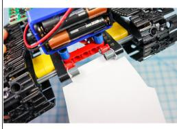
Use two pin/beam sets to connect the paper to the back of the tank under the battery pack where shown.
