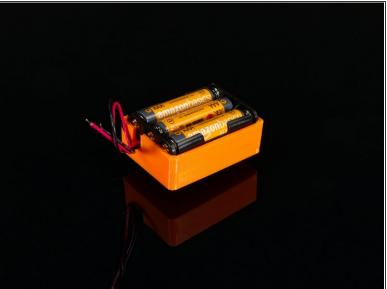
The battery pack sits inside the holder loosely. If you want a more secure fit you can add some tape to hold the battery pack in place.
