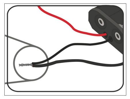
• Twist the Black wire from the Solar Cell together with the Black Wire from the Battery Holder.
