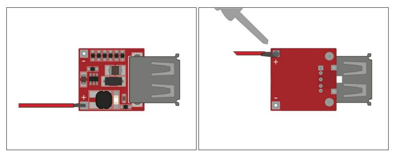
• Solder the Red wire coming off the Switch to the (+) Positive terminal on the USB Circuit.
