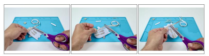
• Measure and cut the three Maker Tape pieces pictured in the photos at left. These pieces will make up the path leading from the pair of Short LED Legs to the negative side of your battery.
