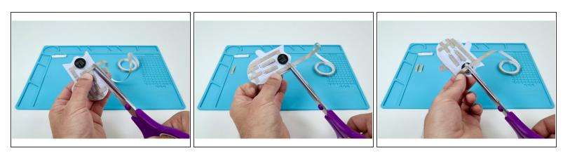
• Measure and cut three final pieces of Maker Tape as shown in the photos at left. These pieces will be used to create the path leading from the Long LED Legs back to the top of the battery.
