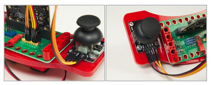
If you're building the <u>Rover Thumbstick Remote</u> the new ribbon cable makes it much easier to get everything plugged into the correct position.
